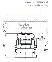
It is permissible to use the C360A/150, C360A/300 and C360A/500 series without arc chamber cover, taking into account additional clearance dimensions. • C360S/... w/o arc chamber
