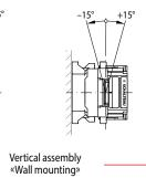
The contactors can be mounted horizontally or vertically on a prepared mounting plate.
