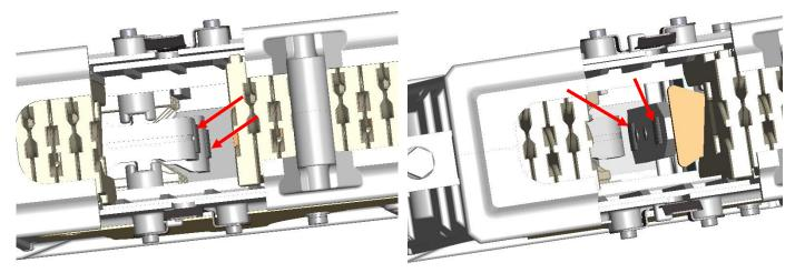
It requires some experience to evaluate the state of the contacts. Even after only a few switchings under load the contacts look used and "dirty" for the inexperienced eye. Contacts need only to be replaced if the wear of the contact tips is more than 70% (less than 0.3 mm remaining).
