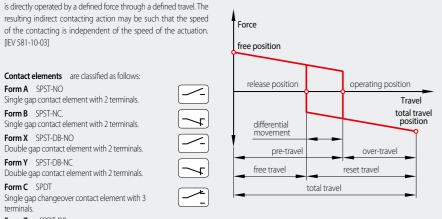
Pre-travel maximum actuator travel between free position and operating position during which there is no movement of the contact elements
